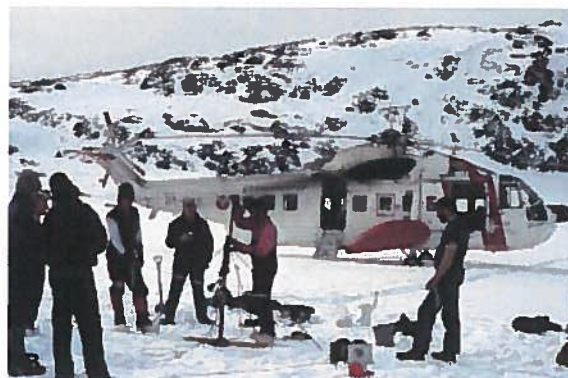
Fig. 3. A: Field camp near one of the lakes in April, 1998. B: The Nesje corer is lifted out of the sediment using a hi-lift jack.
